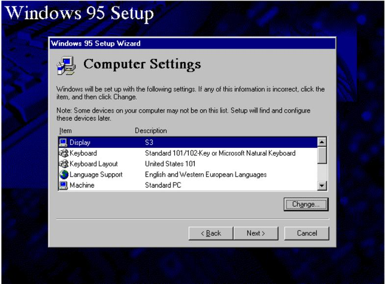
5. □ Setup automatically detects the “Display” with an “S3” display adapter type. Click “Change” and the selections for the display adapter appear as shown in the following figure.
