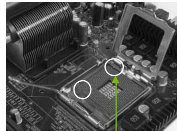
Align notches with notches on the CPU
