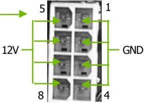
Connect a four-pin power plug to pins 1, 2, 5, and 6.
