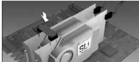
Install the SLI connector onto the two outer cards.
