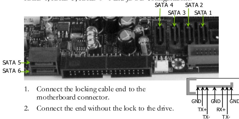
1. Connect the locking cable end to the motherboard connector.
