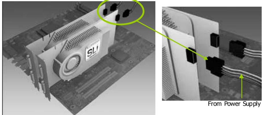
3. Install the NVIDIA SLI connector across the two outer graphics cards as shown below. Each SLI-Ready graphics card has an SLI *finger* on the upper side of the card.
