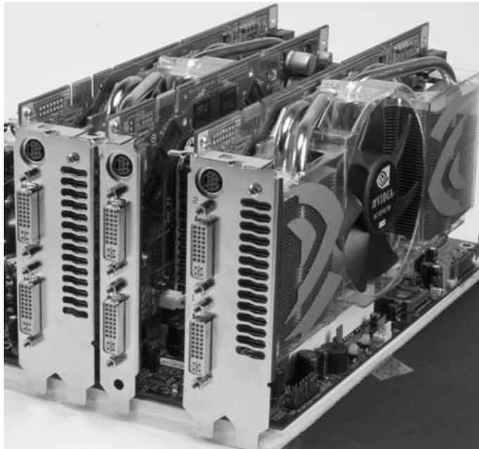
Three PCI Express graphics cards installed. Only the two outer cards will be SLI'ed using the SLI Connector shipped in your motherboard kit.
