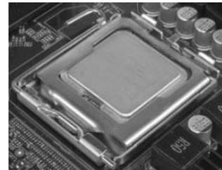
7. Close the load plate over the CPU and press down while you close and engage the socket lever.
