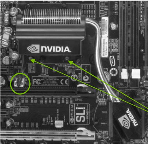
The nForce SPP and MCP have a passive heat sink that draws heat from the chips. You can install a fan onto the SPP heat sink that helps to cool the chips. Hook the fan over the SPP heat sink. Use the two screws to secure the fan to the SPP. Plug the cable into the fan connector.
