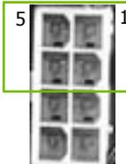
It is *strongly* recommended that you use an 8-pin ATX 12V power supply; however, if you have a four-pin power supply, plug the connector to pins 1, 2, 5, and 6 as shown.
