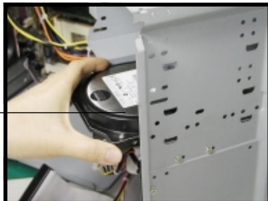
3. Push the drive into the bay until its screw holes align with the holes on the bay marked HDD.
