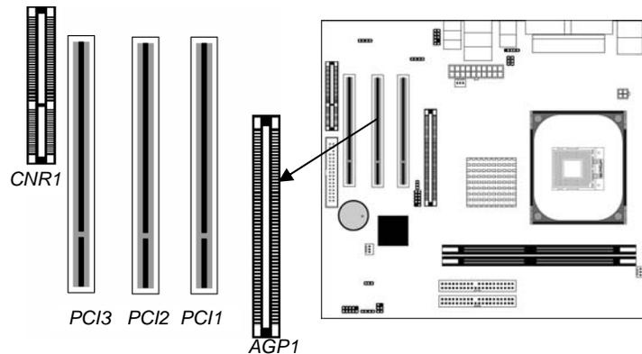
Follow the steps below to install an AGP/CNR/PCI expansion card.
