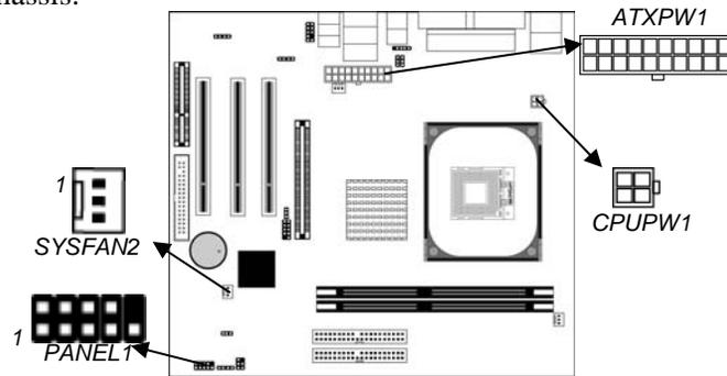
Connect the power connector from the power supply to the **ATXPW1** connector on the mainboard. **CPUPW1** is the CPU Vcore power connector.
