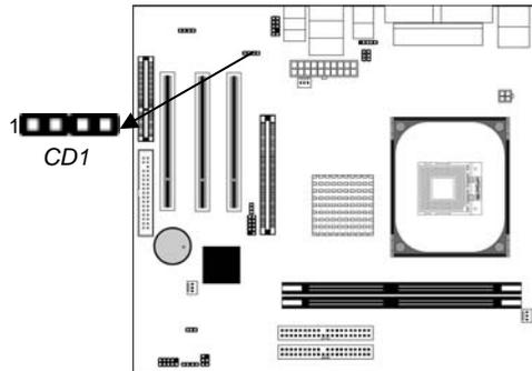
When you first start up your system, the BIOS should automatically detect your CD-ROM/DVD drive. If it doesn't, enter the Setup Utility and configure the CD-ROM/DVD drive that you have installed. On the mainboard, locate the 4-pin connector **CD1**.
