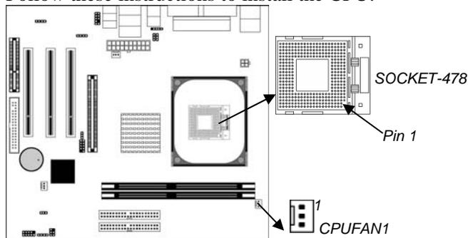
1. Unhook the locking lever of the CPU socket. Pull the locking lever away from the socket and raising it to the upright position.
