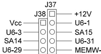
Figure 2. Expansion Socket Configuration Options
