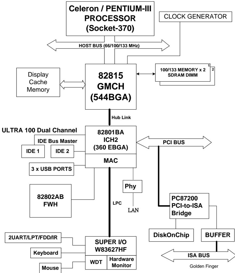
**Figure 1-1 ROBO-679 System Block Diagram**
