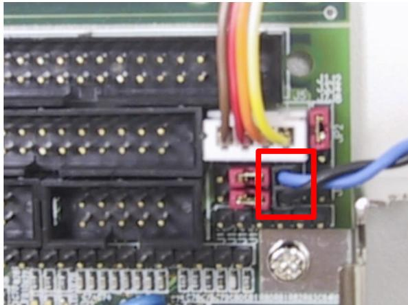
Step6: The figure below is the TOGGLE SWITCH, which is used to switch the ATX Power on/off for SBC. Usually the TOGGLE SWITCH is located on the chassis front panel. By pressing the switch button once, the power will be on, and press again to turn it off.
