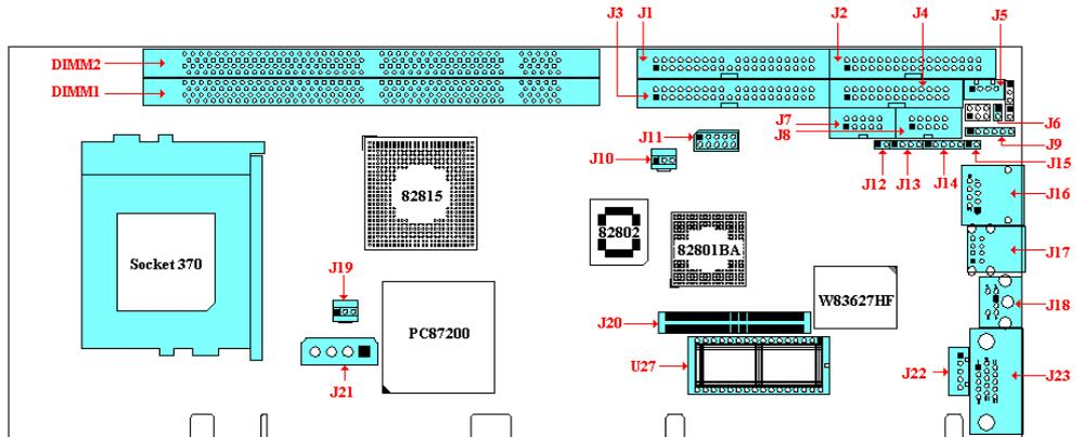
**Figure 2-2 ROBO-679 Connector Locations**
