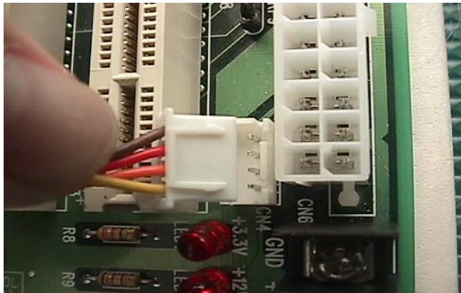
Step4: Please find the J5 4-pin header on the center part of ROBO-679 in white color. You will also see a mark with "J5" at the right top corner of J5 header. Connect the 4-pin power control cable with this J5 header.
