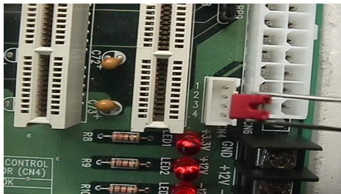
Step2: Connect 20-pin power cable of the ATX POWER with the CN7 (ATX POWER CONNECTOR, 20-pin) connector on the backplane. The CN7 is located on the upper-right side of the backplane with white color.
