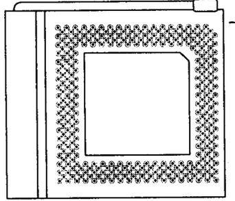
Figure 1 Socket 7 for Pentium CPU
