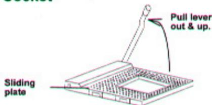
2. Align the CPU and socket pin 1 corners. The pins on the bottom should align with the inner 3 rings of holes in the socket, then place the CPU in the socket. It should insert easily. If it doesn't, pull the level up a little more.
