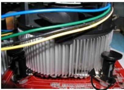
9. Gently rotate the cap clockwise 1/4 turn to fasten the heatsink onto the Sapphire motherboard.
