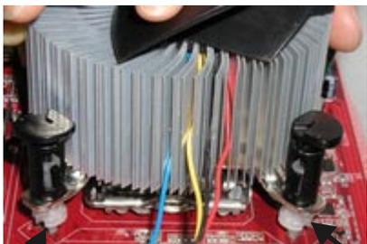
7. Align the fastener tips with the motherboard hole pattern, insert the fastener tips into the holes, guiding the wires to avoid pinching. The fasteners will slide through the Sapphire motherboard holes without applying too much force.
