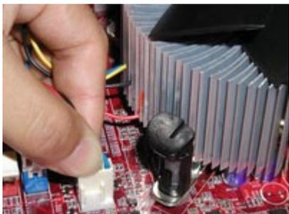
10. Lastly, attach the fan wire connector to the 4 pin fan header connector on the Sapphire motherboard labeled CPU FAN.
