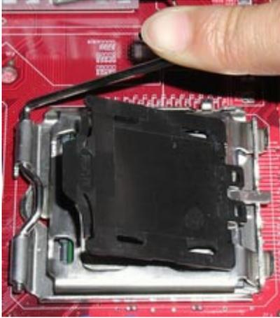
4. Use index finger and thumb to press down the metal lever. The cap will be pushed up by the CPU. This may also be done by removing the lid beforehand.
