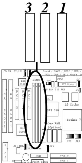
The DIMM types supported SDRAM (Synchronous DRAM). The following is the summary:
