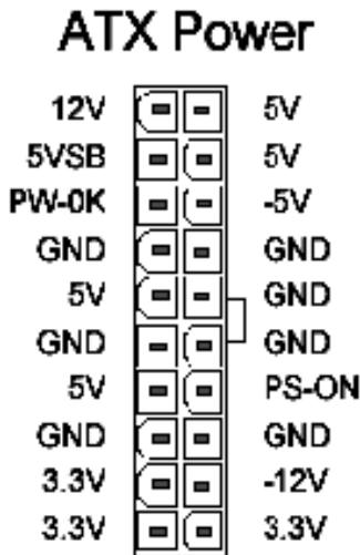
Make sure that your ATX power supply can supply at least 10 mAmp on the 5-volt standby lead (5VSTB). You may experience difficulty in powering on your system if your power supply cannot support the load. For Wake on LAN support, your ATX power supply must supply at least 1 Amp.
