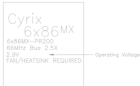
Fig. 2g CPU Description (Top Side)
