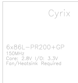
Fig. 2f CPU Description (Top Side)
