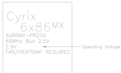
Fig. 2g CPU Description (Top Side)
