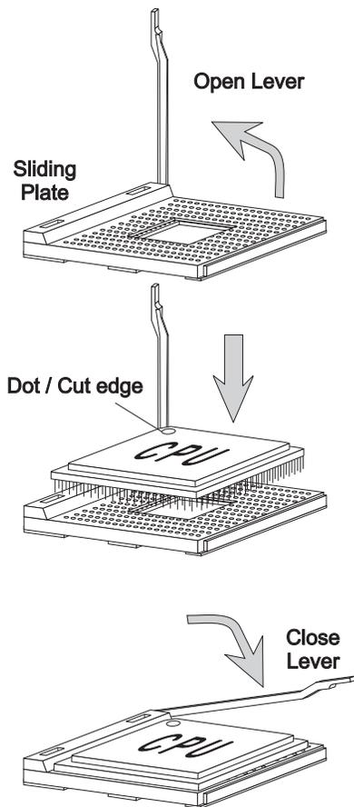
1. Pull the lever sideways away from the socket. Then raise the lever up to a 90-degree angle.
