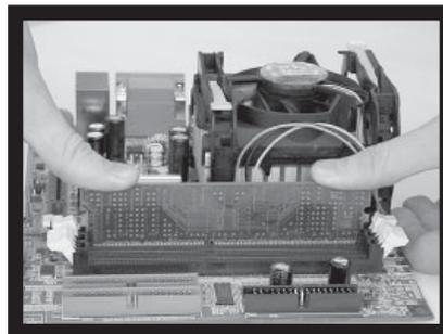
3. The plastic clips at sides of the DIMM slot will automatically close shut.
