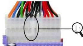
With ATX v2.x power supply, users please note that when installing 24-pin power cable, the latches of power cable clings to the right side of the ATX1 connector latch.
