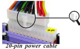
With ATX v1.x power supply, users please note that when installing 20-pin power cable, the latch of power cable clings to the left side of the ATX1 connector latch, just as the picture shows.
