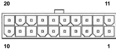
This connector (ATXR1) supplies the CPU operation voltage (Vcore), be sure to insert below power connector in your motherboard.
