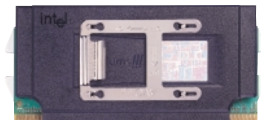
Example of an incorrectly installed retention clip
