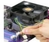
**Note 1:** To achieve better airflow rates and heat dissipation, we suggest that you use a high quality fan with 3800 rpm at least. CPU fan and heatsink installation procedures may vary with the type of CPU fan/ heatsink supplied. The form and size of fan/heatsink may also vary.
