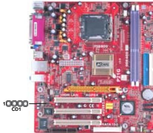
When you first start up your system, the BIOS should automatically detect your CD-ROM/DVD drive. If it doesn't, enter the Setup Utility and configure the CD-ROM/DVD drive that you have installed. On the motherboard, locate the 4-pin header **CD1**.
