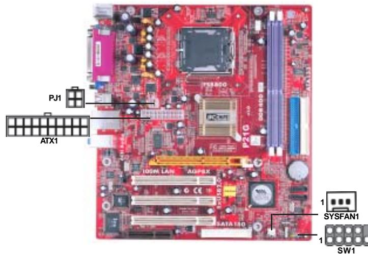
Connect the power connector from the power supply to the **ATX1** connector on the motherboard. The **PJ1** is a +12V connector for CPU Vcore power.
