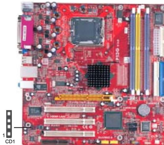
When you first start up your system, the BIOS should automatically detect your CD-ROM/DVD drive. If it doesn't, enter the Setup Utility and configure the CD-ROM/DVD drive that you have installed. On the motherboard, locate the 4-pin header **CD1**.
