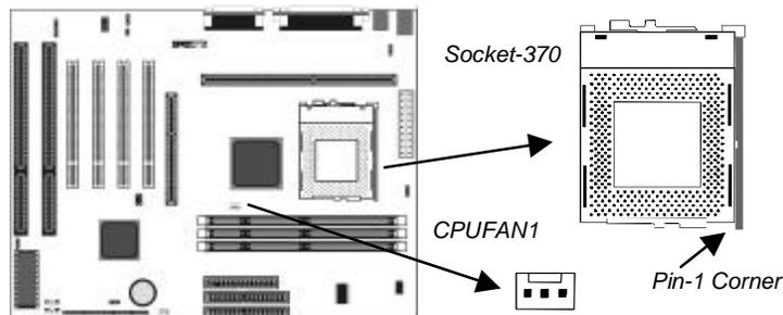
2. On the Celeron processor, identify the pin-1 corner by noting that it has a slight bevel.
