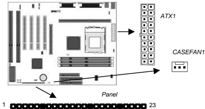
Connect the power cable from the power supply unit to the power connector ATX1 on the mainboard. If the system chassis is installed with a cooling fan, connect the cable from the cooling fan to the chassis fan power connector on the mainboard CASEFAN2.
