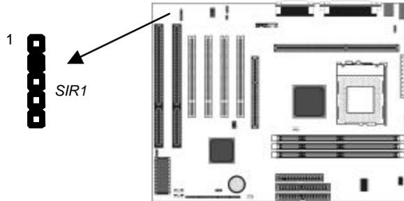
1. On the mainboard locate the infrared port header SIR1.
