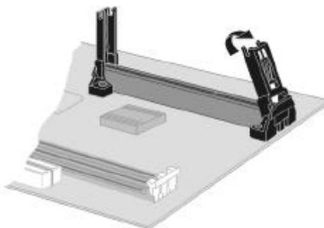
3. Insert the processor cartridge into the cartridge holder. Follow the instructions given with your processor cartridge. The edge connector on the cartridge has a notch so that it only fits into the Slot-1 in the correct way.
