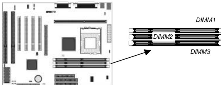
For this mainboard, you must use 168-pin, 3.3V memory modules installed with SDRAM memory chips. If you are using a processor cartridge that runs on a 100 MHz system bus, you must use memory that operates on a 100 MHz memory bus (PC-100 memory). If you are using a processor cartridge that runs on a 66 MHz system bus, you can use memory that operates on a 66 MHz memory bus.
