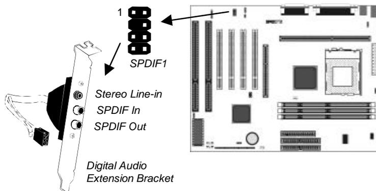
1. On the mainboard, locate the SPDIF1 header for this bracket.
