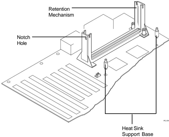
Push the Heat Sink Support Base onto the mainboard, until you hear a click sound. Check for a perfect fit.
