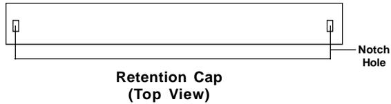
To remove the Retention Cap, you need a Screw Driver (0.3 cm) tip.
