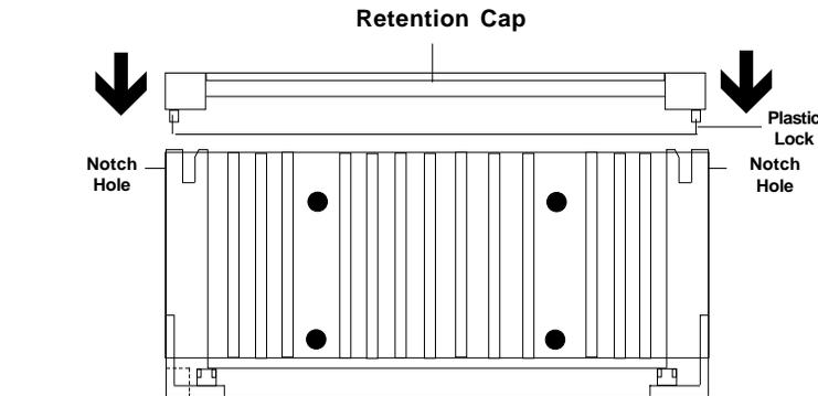
Lock the processor by putting the Retention Cap provided. Take note of the two plastic lock at the side of the Retention Cap. This two plastic lock should be aligned properly into the Retention Mechanism notch hole.
