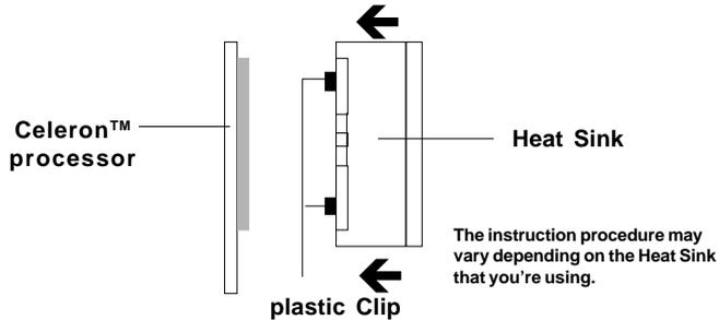
Push down the plastic clips, so that they are in line with the hole on the processor. Check for perfect fit.
