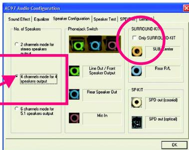
When the "Environment settings" is "None", the sound would be performed as stereo mode (2 channels output). Please select the other settings for 4 channels output.
