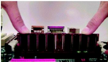
1. The DIMM socket has a notch, so the DIMM memory module can only fit in one direction.
