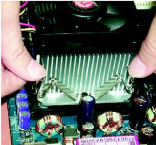
1. Fasten the cooling fan supporting-base onto the CPU socket on the mainboard.
