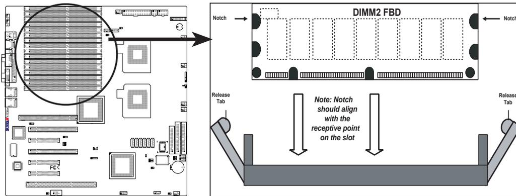
**To Install:** Insert module vertically and press down until it snaps into place. Pay attention to the alignment notch at the bottom.
