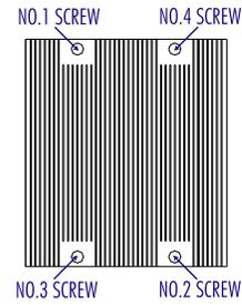
2. Hold the heatsink as shown in the picture on the right and gently wriggle the heatsink to loosen it from the CPU. (Do not use excessive force when wriggling the heatsink!!)
