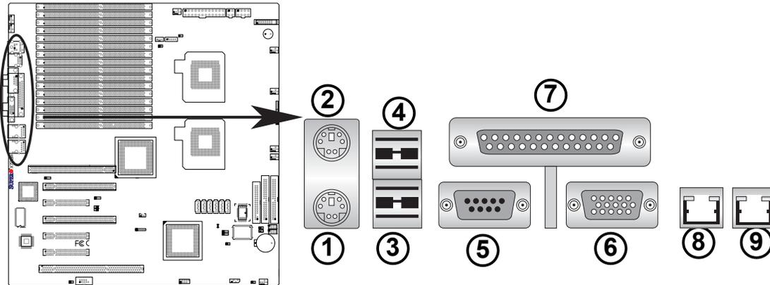
**Figure 2-3. Back Panel I/O Port Locations and Definitions**
