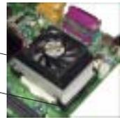
9. Secure the heat sink by locking the retention clips into their proper position.
