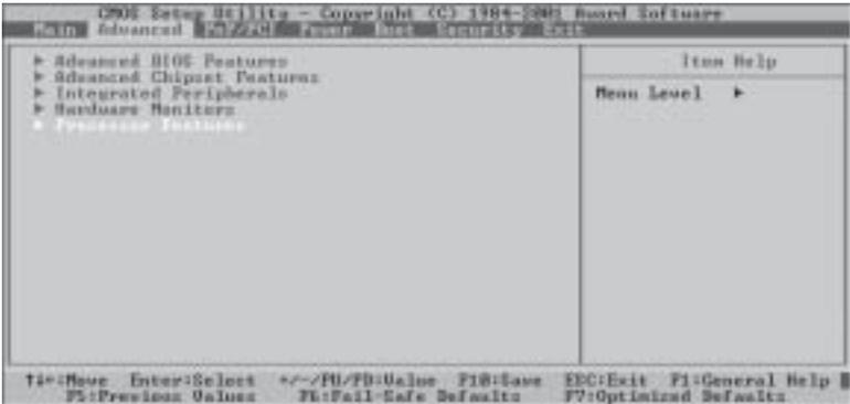
When the item "Processor Features" is highlighted, hit the <Enter> key to activate the sub-menu, which is shown below.
