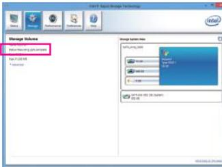
The **Status** item on the left of the screen displays the rebuild progress.
