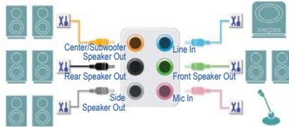
For example, in a 4-channel audio configuration, if a Rear speaker is plugged into the default Center/Subwoofer speaker out jack, you can retask the Center/Subwoofer speaker out jack to be Rear speaker out.
