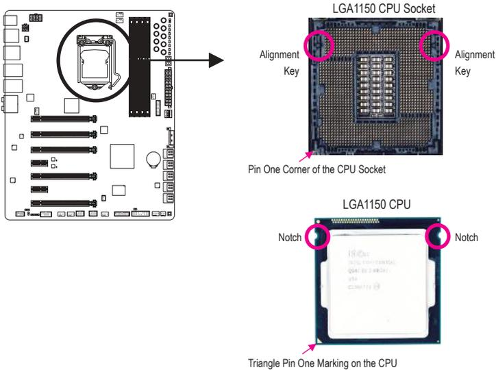
B. Follow the steps below to correctly install the CPU into the motherboard CPU socket.
