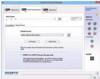
(Note) Enter the **Digital Output(Optical)** screen to configure further settings if you use the S/PDIF Out connector(s) on the back panel for digital audio output or enter the **Digital Output** screen if you use the internal S/PDIF Out connector (SPDIF\_O) for digital audio output.
