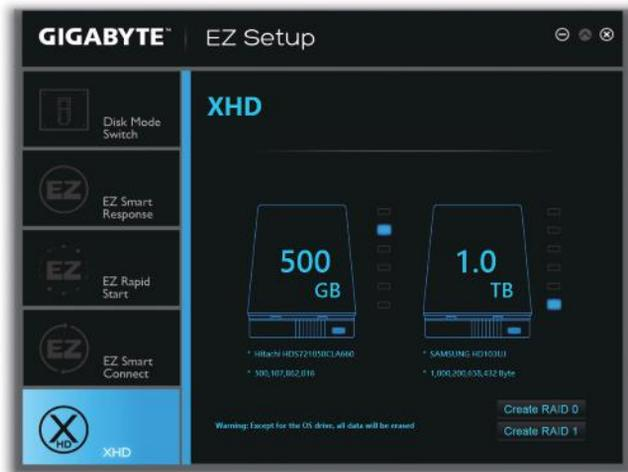
(Note 1) The XHD utility only supports the SATA connectors controlled by the Intel® Chipset.
