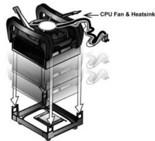
6. Flip the levers over to lock the heat sink in place.
