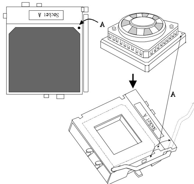
1. Pull the lever sideways away from the socket then raise the lever up to a 90-degree angle.
