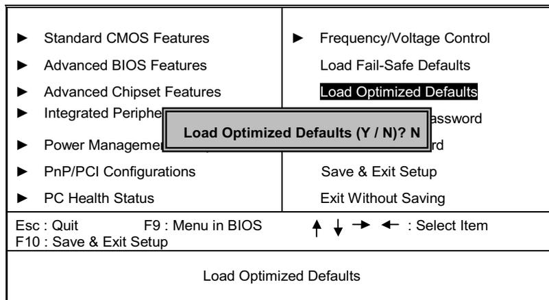
Pressing 'Y' loads the default values that are factory settings for optimal performance system operations.
