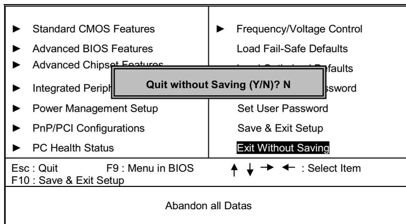
Type "Y" will quit the Setup Utility without saving to RTC CMOS RAM.
