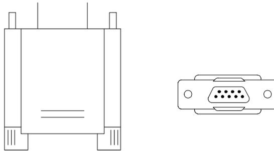
The serial port on this system has one 9-pin connector. Some older computer systems and peripherals used to be equipped with only one 25-pin connector. Should you need to connect your 9-pin serial port to an older 25-pin serial port, you can purchase a 9-to-25 pin adapter.
