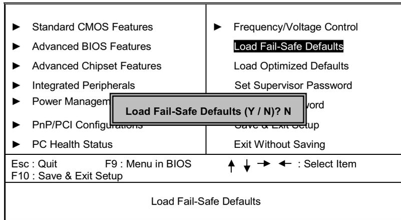
Pressing 'Y' loads the default values for the most stable, minimal performance system operations.
