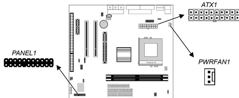
Connect the power connector from the power supply to the **ATX1** connector on the mainboard.
