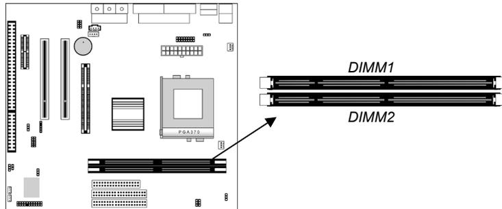
For this mainboard, you must use 168-pin, 3.3V unbuffered PC100 or PC133 SDRAM memory modules. You can install any size memory module from 16 MB to 512MB, so the maximum memory size is  $2 \times 512\text{MB} = 1\text{GB}$ .
