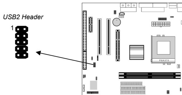
1. Locate the **USB2** header on the mainboard.
