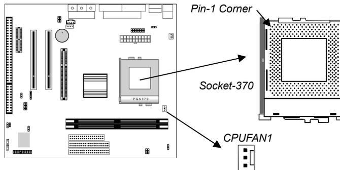
2. On the processor, identify the Pin-1 corner by its beveled edge.
