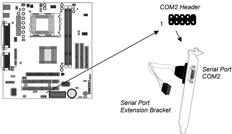
1. On the mainboard, locate the header COM2 for this bracket.
