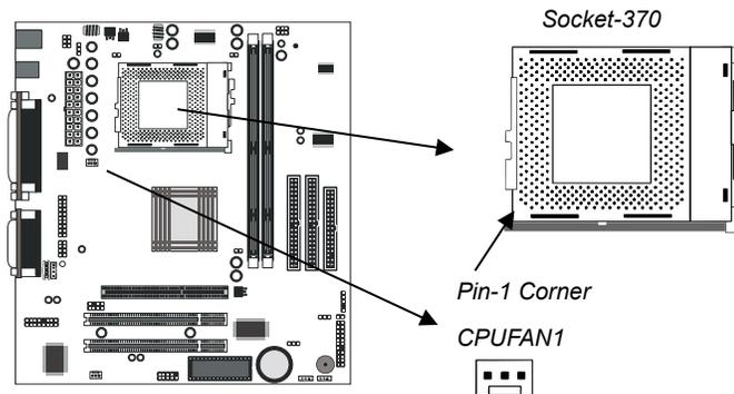
2. On the processor, identify the Pin-1 corner by its beveled edge.
