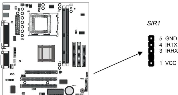
1. Locate the infrared port SIR1 header on the mainboard.
