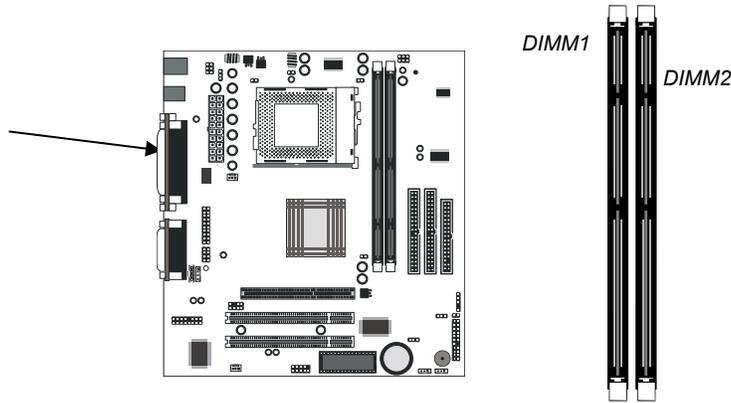
For this mainboard, you must use 168-pin, 3.3V unbuffered SDRAM memory modules. If the installed CPU uses a 100MHz system bus, you must use PC100 or PC133 memory. If the installed CPU uses a 66MHz system bus, you must use PC66 memory. You can install any size memory module from 16 MB to 512MB, so the maximum memory size is  $2 \times 512\text{MB} = 1\text{GB}$ .
