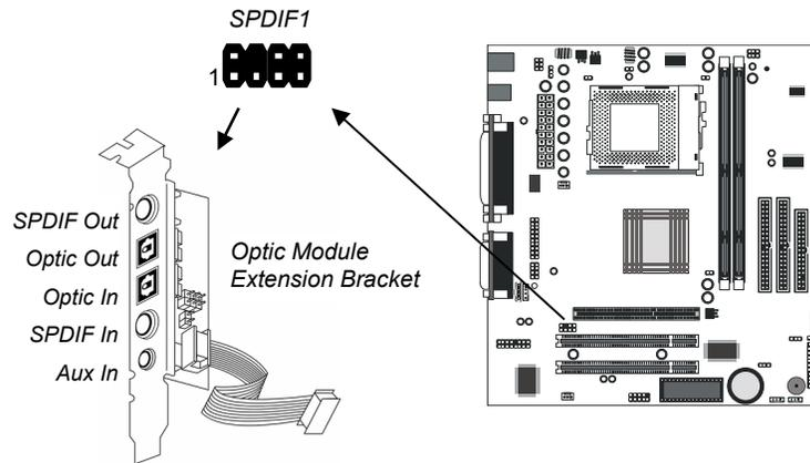
1. On the mainboard, locate the SPDIF1 header for this bracket.
