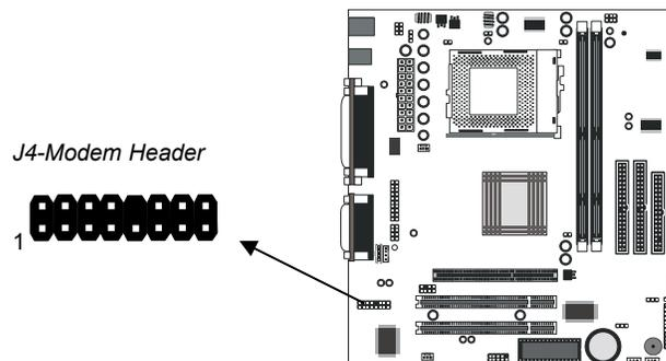
1. Locate the J4 modem header on the mainboard.
