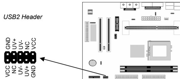
1. Locate the **USB2** header on the mainboard.
