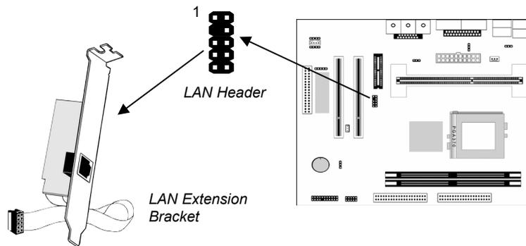
1. On the mainboard, locate the LAN header for this bracket.
