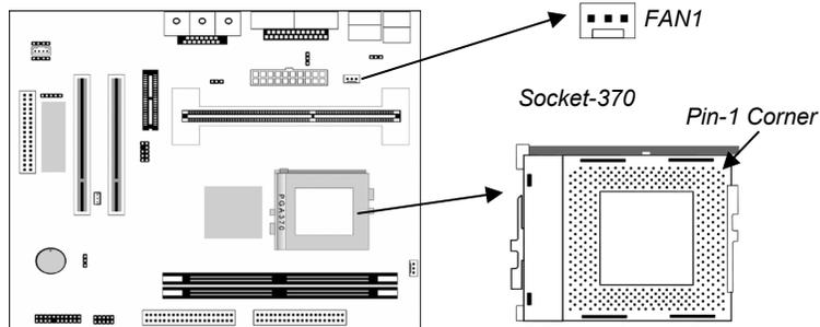
2. On the processor, identify the Pin-1 corner by its beveled edge.
