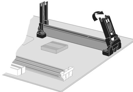
3. Slide the CPU cartridge into the module arms. Follow the instructions that come with the CPU. The edge connector on the CPU cartridge has a notch so that it only fits into the Slot-1 in the correct way.
