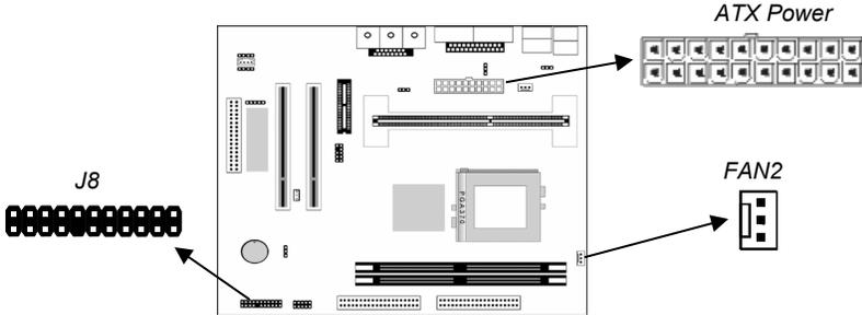
Connect the power connector from the power supply to the **ATX** Power connector on the mainboard. If there is a cooling fan installed in the system chassis, connect the cable from the cooling fan to the **FAN2** fan power connector on the mainboard. Connect the case switches and indicator LEDs to the **J8** switch and LED connector header. See the illustration below for a guide to the J8 connector pin assignments.
