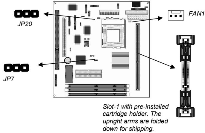
2. The Slot-1 is installed with a cartridge holder. The upright struts of the cartridge holder are folded down for shipping. Pull the struts upwards so that they are in the upright position.
