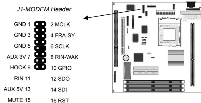
1. Locate the J1 modem header on the mainboard.
