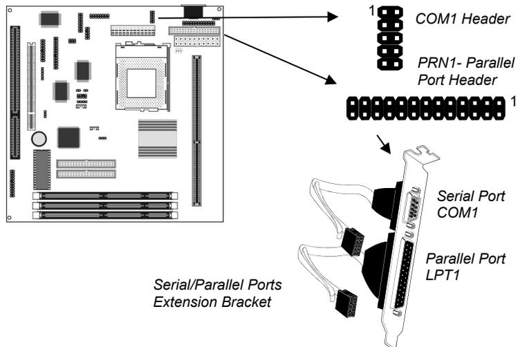
1. On the mainboard, locate the headers COM1 and PRN1 for this bracket.
