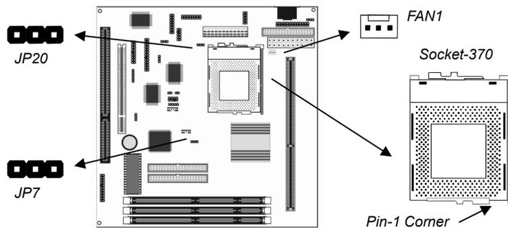
2. On the processor, identify the pin-1 corner by noting that it has a slight bevel.
