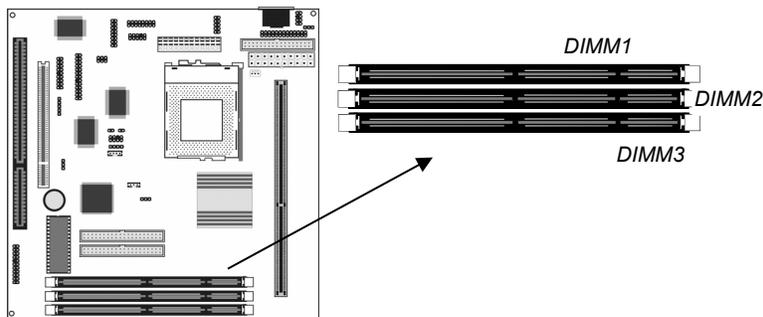
For this mainboard, you must use 168-pin, 3.3V memory modules installed with SDRAM memory chips. If you are using a processor cartridge that runs on a 100 MHz system bus, you must use memory that operates on a 100 MHz memory bus (PC-100 memory). If you are using a processor cartridge that runs on a 66 MHz system bus, you can use memory that operates on a 66 MHz memory bus. You can install any size of memory module from 16 MB up to 256 MB, so the maximum memory size is 3 x 256 MB = 768 MB.
