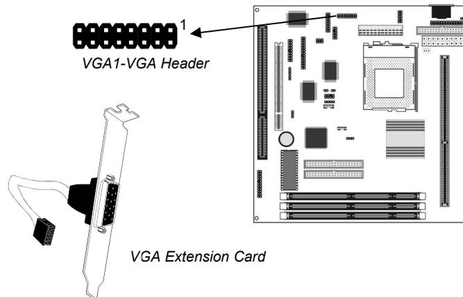
1. On the mainboard, locate the VGA1 header for this bracket.
