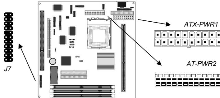
Connect the power cable from the power supply unit to the power connector on the mainboard. If you are using an AT power unit, connect it to the AT power connector PWR2. If you are using an ATX power unit connect it to the ATX power connector PWR1.
