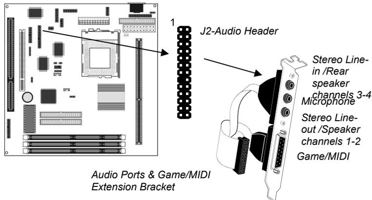
1. On the mainboard, locate the J2 audio header for this bracket.
