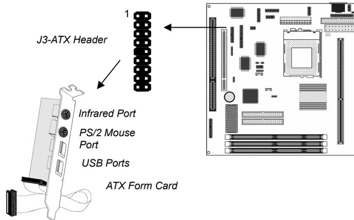
1. On the mainboard, locate the J3 ATX header for this bracket.
