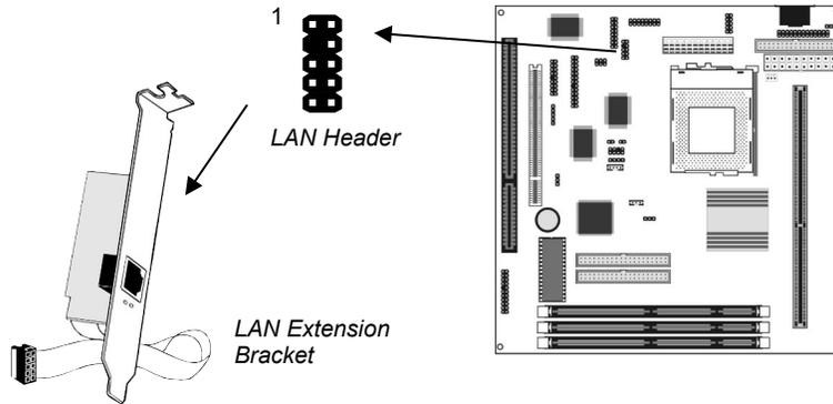
1. On the mainboard, locate the LAN1 header for this bracket.
