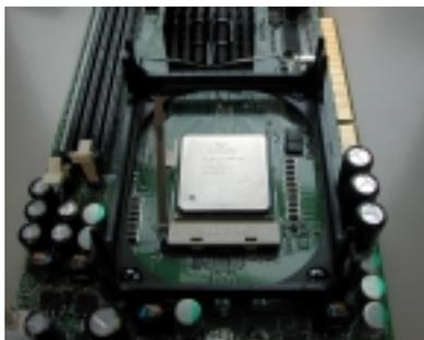
**Step3:** Push the lever down to close the socket.
