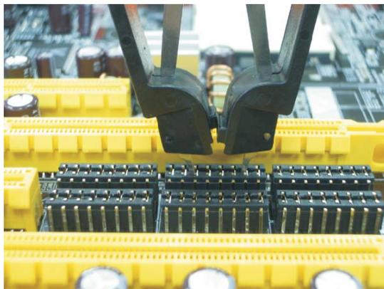
This will easily remove the jumper cap.
