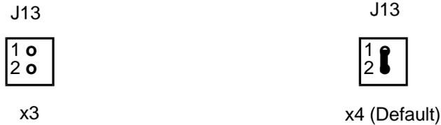
**NOTE : WinSystems warrants the operation and reliability of the LPM/MCM-DX5-133 only in the 33x4 mode. Any other jumpering may not result in reliable operation.**
