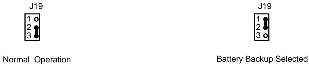
**NOTE :** Having the jumper selected for battery backup when using anything other than low-power-standby SRAMs (such as with EPROMs, or PEROMs) will result in the rapid draining of the onboard battery.
