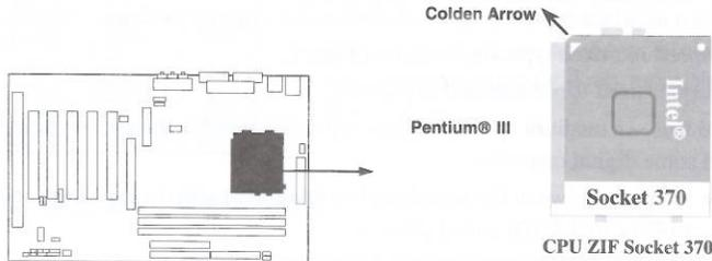
When you put the CPU into the ZIF socket. No force require to insert of the CPU, then press the level to Locate position slightly without any extra force.
