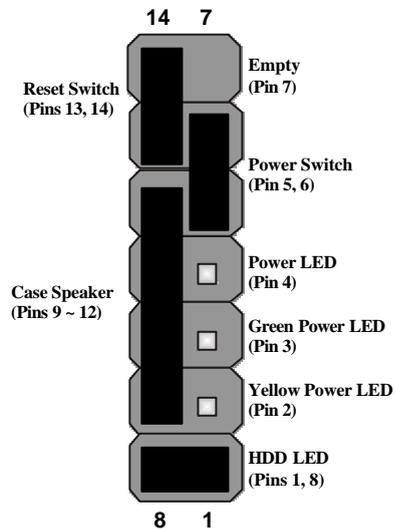
**Note:** The plus sign (+) indicates a pin which must be connected to a positive voltage.
