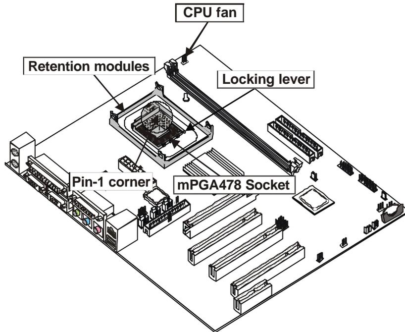
**Note:** The pin-1 corner is marked with an arrow ▼
