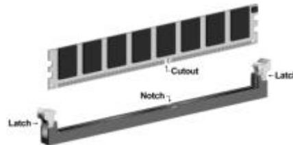
5. Check that the cutouts on the DIMM module edge connector match the notches in the DIMM slot.
