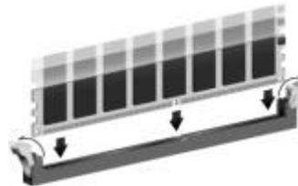
6. Install the DIMM module into the slot and press it firmly down until it seats correctly. The slot latches are levered upwards and latch on to the edges of the DIMM.
