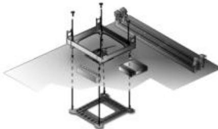
3. Install your CPU. Pull up the lever away from the socket and lift up to 90-degree angle.
