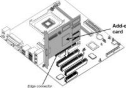
An isometric diagram of a computer motherboard. An add-on card is shown being inserted into an expansion slot. A label 'Add-on card' points to the card, and a label 'Edge connector' points to the gold-plated contacts on the card's edge. The card is partially inserted into the slot, with its metal bracket resting on the motherboard's surface. |
