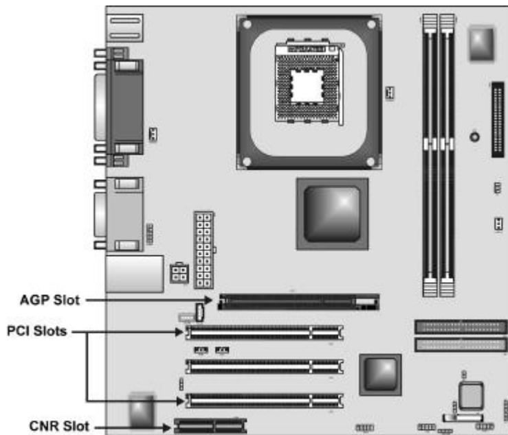
**PCI Slots** PCI slots are used to install expansion cards that have the 32-bit PCI interface.
