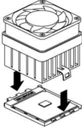
A line drawing showing a square CPU cooling fan/heatsink assembly being lowered onto a CPU socket. Two black arrows point downwards from the assembly towards the socket, indicating the direction of movement.               |
