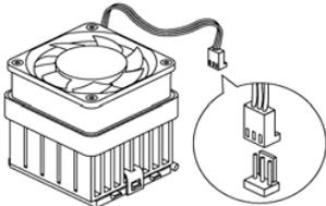
A line drawing of the CPU cooling fan/heatsink assembly. A power cable is connected to the fan. A circular inset shows a close-up of the power cable connector being inserted into the CPUFAN connector on the motherboard. |
