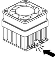
A line drawing of the CPU cooling fan/heatsink assembly. Two black arrows point to the retention clips on either side of the fan/heatsink unit, indicating where they should be secured onto the Socket 462 base.            |
