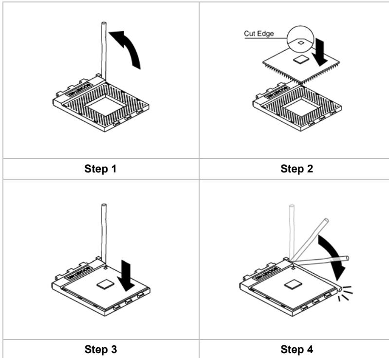
Orient the CPU so the odd corner matches the odd corner of the socket. With the lever in an upright position, gently place the CPU on the socket; make sure that all pins line up with the socket holes. When pins are aligned, the CPU should seat itself in the socket. Apply very light pressure to ensure the CPU is evenly seated. Push the lever down and ensure it latches firmly.
