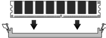
4. Check that the cutouts on the DIMM module edge connector match the notches in the DIMM slot.
