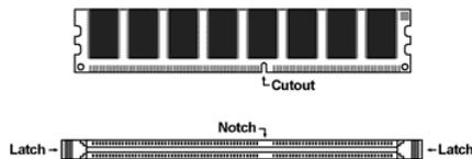
2. Push the latches on each side of the DIMM slot down.
