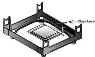
6. Apply thermal grease on top of the CPU.
