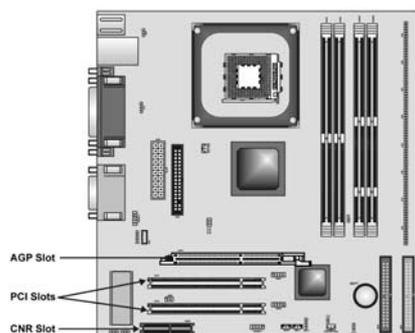
**PCI Slots** PCI slots are used to install expansion cards that have the 32-bit PCI interface.
