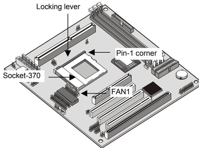
1. On the mainboard, locate the socket-370 and FAN1.
