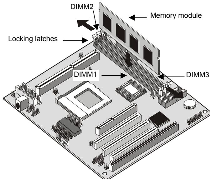
2. The DIMM slots are keyed with notches and the DIMMs are keyed with cut-outs so that they can only be installed correctly. Check that the cut-outs on the DIMM module edge connector match the notches in the DIMM slot.
