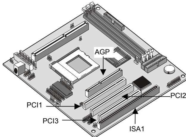
1. Before installing an expansion card, check the documentation for the card carefully. If the card is not Plug and Play, you may have to manually configure the card before installation.
