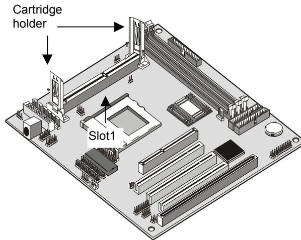
If the cartridge holder is not already installed, install it onto the slot1. Some cartridge holders are in two parts, one part for each end of the slot1. Other cartridge holders are a single assembly that sits over the whole length of the slot1.
