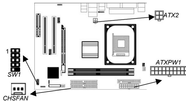
Connect the power connector from the power supply to the **ATXPW1** connector on the mainboard. **ATX2** is the CPU Vcore power connector.
