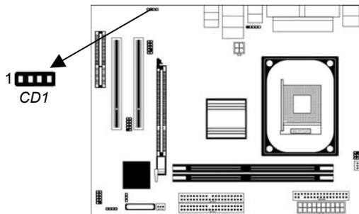
When you first start up your system, the BIOS should automatically detect your CD-ROM/DVD drive. If it doesn't, enter the Setup Utility and configure the CD-ROM/DVD drive that you have installed. On the mainboard, locate the 4-pin connector **CD1**.
