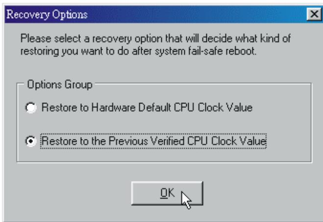
c. "Auto-overclock button": User can click this button and [ WarpSpeeder™ ] will set the best and stable performance and frequency automatically. [ WarpSpeeder™ ] utility will execute a series of testing until system fail. Then system will do fail-safe reboot by using Watchdog function. After reboot, the [ WarpSpeeder™ ] utility will restore to the hardware default setting or load the verified best and stable frequency according to the Recovery Dialog's setting.
