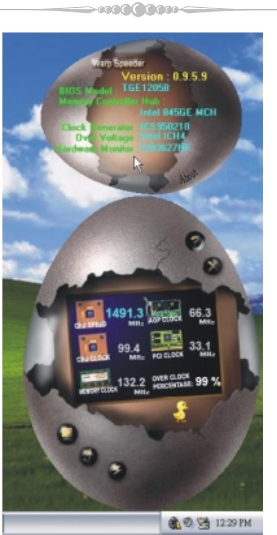
Note: Because the overclock, overvoltage, and hardware monitor features are controlled by several separate chipset, [ WarpSpeeder™ ] divide these features to separate panels. If one chipset is not on board, the correlative button in Main panel will be disabled, but will not interfere other panels' functions. This property can make [ WarpSpeeder™ ] utility more robust.
