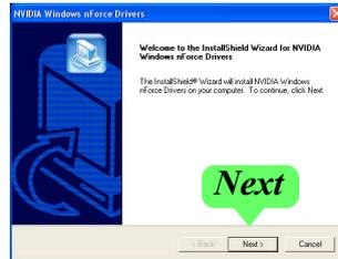
3. The nVIDIA InstallShield Wizard will pop up to guide you to set up nForce3 Drivers. This All-in-1 Driver will first start to install GART Driver.
