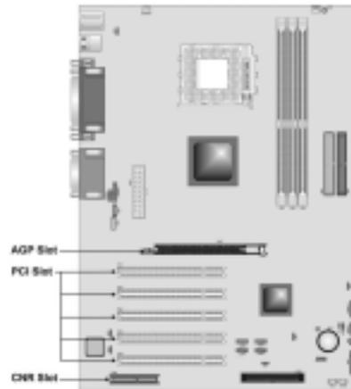
**Note:** Before installing an add-on card, check the documentation for the card carefully. If the card is not Plug and Play, you may have to manually configure the card before installation.
