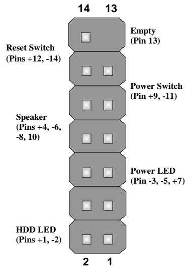
**Note:** The plus sign (+) indicates a pin which must be connected to a positive voltage.
