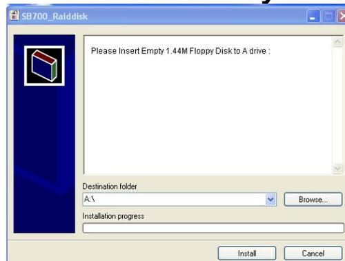
2. Copy the files to floppy disk and restart the computer with floppy disk as the first booting disk and then follow the steps shown on the screen to finish RAID function settings.
