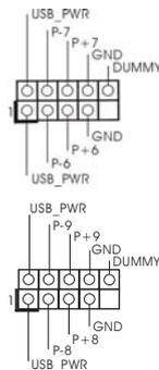
Besides six default USB 2.0 ports on the I/O panel, there are two USB 2.0 headers on this motherboard. Each USB 2.0 header can support two USB 2.0 ports.
