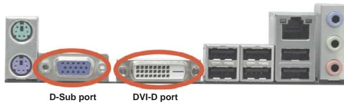
2. If you have installed onboard VGA driver from our support CD to your system already, you can freely enjoy the benefits of dual monitor function after your system boots. If you haven't installed onboard VGA driver yet, please install onboard VGA driver from our support CD to your system and restart your computer.
