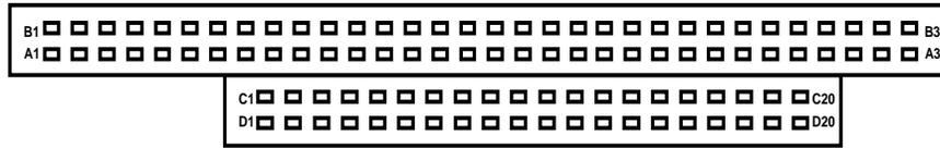
Drawing of PC104 pin header
