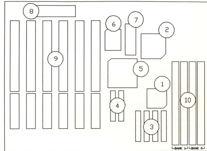
Fig 1 Key Components of the GMB-386SOP Mainboard
