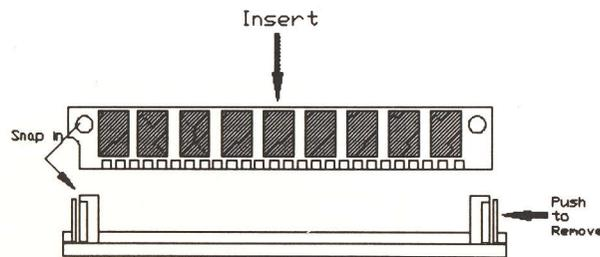
Fig 6 Installing a SIMM
