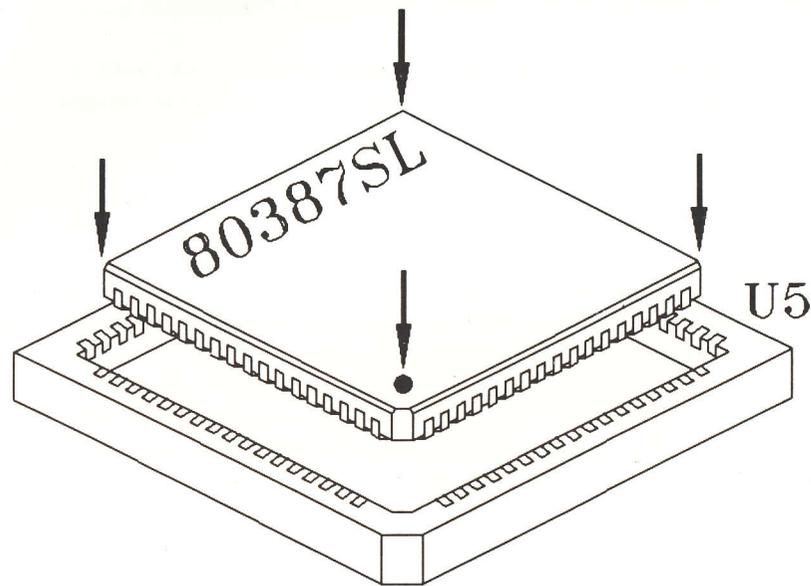
Fig 3 Installing an 80387SL Coprocessor
