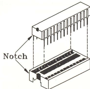
Fig 5 Installing a Cache Chip
