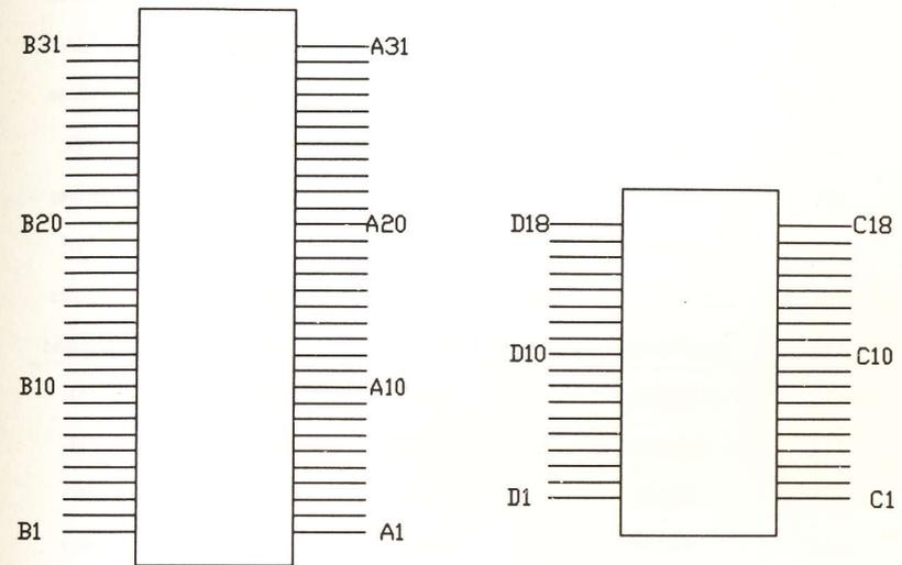
Fig 8 16-bit Channel Pin Assignments
