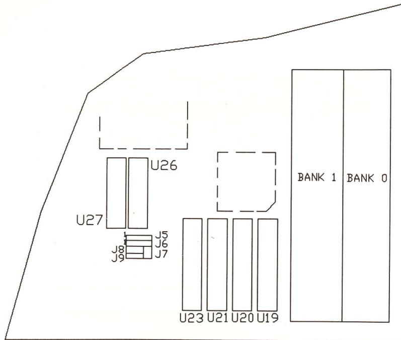
Fig 4 Cache Jumper and Socket Locations
